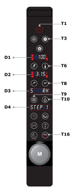
Once the oven has been switched on by pressing the **T1** key, select the steaming mode by pressing the **T3** key. Activate the desired cooking temperature setting by pressing the **T6** key, signalled by the flashing of the key itself: set the temperature value by acting on the **M** knob (up to 120°C) and confirm the selection by pressing the **T6** key or the **M** knob ofthe encoder.
