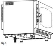
Connect the oven to the gas supply using a special R 1/2'' hose with an internal section of at least 16 mm. Connection to gas supply must be carried out using rigid or flexible metal pipes.
