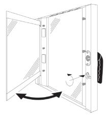
The door glass can be cleaned externally and internally. For this purpose, turn the stop holding the internal glass in position clockwise and, once the glass is opened, clean it with suitable detergent.
