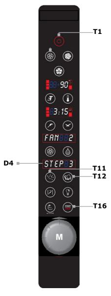
To access a memorised program, press the **T12** Book key and select the program number, shown on the **D4** display, by turning the **M** knob to right or to left.Confirm the selection by pressing the **M** knob when the disired program nuber is shown on the **D4** display.
