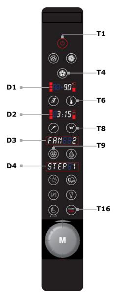
Once the oven has been switched on by pressing the **T1** key, select the convection/steam mixed cooking modality by pressing the **T4** key.
