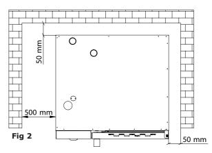
between the oven and the walls or other equipment. It is advisable to leave 500 mm space between the left side of the oven and the corresponding wall of the room (**Fig. 2**) to allow the oven to be installed easily and facilitate successive maintenance.
