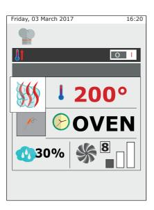
To set the desired level of humidity, press button **7** and set the valve.
