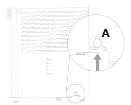
The oven is equipped with a water drain; this device is placed at the bottom of the rear part of the appliance and has a tube with diameter of 32 mm.
