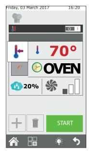
The hold mode has the purpose of maintaining the products at a hygienically safe temperature(> 65°C) without product core cooking undergoing changes. It is used at the end of night time cooking to maintain the products cooked until the operator returns.
