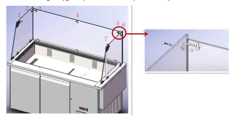
4. Install the top glass by L shape bracket.
